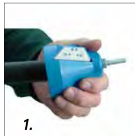
1. Cut the pipe square, the chamfer.
